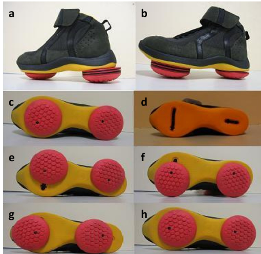
Fig. 2. Calibration of the elements on the base of the biomechanical device: (a) Plantar flexion configuration (hindfoot element elevated); (b) dorsal flexion configuration (forefoot element elevated); (c) neutral sagittal configuration; (d) elements removed; (e) lateral sagittal axis configuration; (f) medial sagittal axis configuration; (g) anterior configuration; (h) posterior configuration. This study presents muscle activity in lateral, medial, anterior, posterior, dorsi and plantar flex configurations only.
