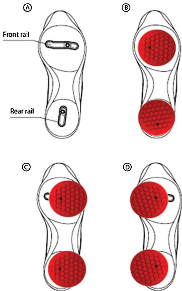
**Figure 2.** (A) Biomechanical device with no elements attached; (B) at neutral sagittal axis; (C): at lateral sagittal axis; and (D): at medial sagittal axis.
