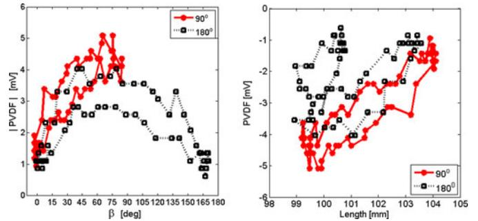
Fig. 9. Examples of PVDF response-loops in different work ranges. Left—PVDF (absolute values) versus deflection angle  $\beta$ . In the limited range ( $\beta < 90^\circ$ ) the PVDF monitors  $\beta$  well but, beyond this range, the PVDF loses any linear correlation to  $\beta$ . Right—examining the PVDF-length loops reveals that the PVDF signal resembles strain more than deflection outside the limited working range.
