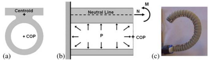
Fig. 1. Bending induced by the cross section's nonaxisymmetric profile. (a) Illustration of a cross section with its compound-beam centroid ( $\bar{x}$ ) and the COP. (b) Side view demonstrating the equivalent tensile force  $N$  and bending moment  $M$  induced by the actuation pressure. (c) Resulting deflection of the bi-bellows actuator.
