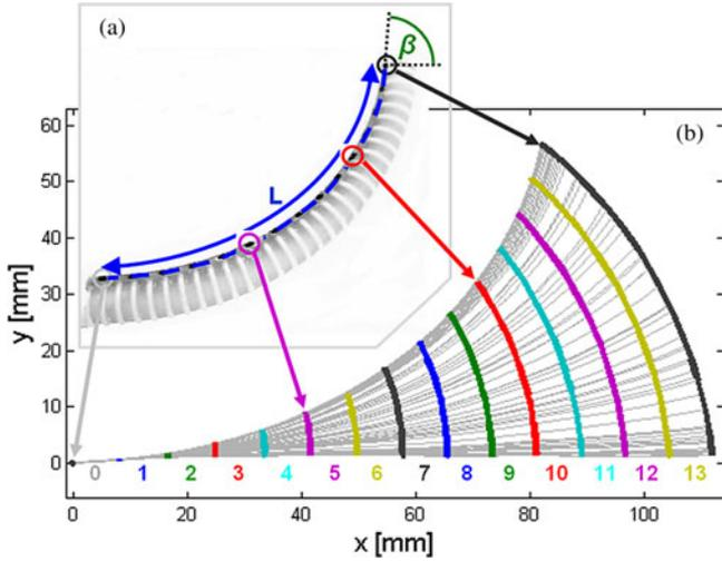
Fig. 6. Visual-tracking demonstration during a single cycle. (a) Snapshot with four tracers circled,  $L$ —actuator length taken along a spline passing through the tracers, and  $\beta$ —the tip angle. (b) Tracer positions during the whole cycle are depicted by thick colored lines. A thin gray spline connects the tracers at each given point in time. The spline segments between each pair of tracers are numbered 0–13 and their length is recorded.
