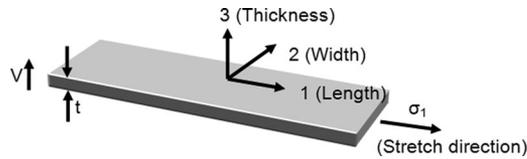
Fig. 2. Notation for a PVDF-film transducer.
