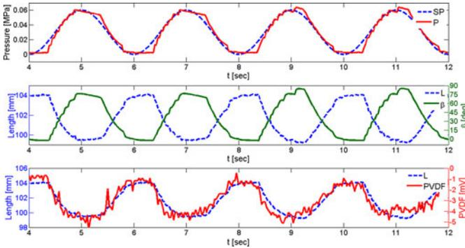
Fig. 7. Actuation trial of a free actuator bent up to  $90^\circ$ . Top—pressure set point (SP, dashed blue) versus the actual pressure measured (P, solid red). Middle—features extracted by visual tracking: actuator length ( $L$ , dashed blue), and tip angle ( $\beta$ , solid green). Bottom—PVDF reading (PVDF, solid red) versus the actuator length ( $L$ , dashed blue).
