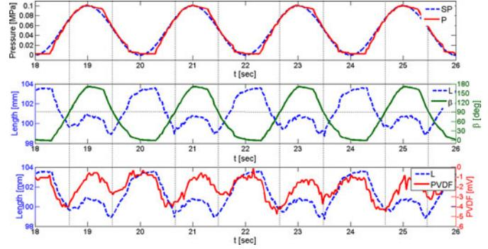
Fig. 8. Actuation trial of a free actuator bent up to  $180^\circ$ . Top—pressure set point (SP, dashed blue) versus the actual pressure measured (P, solid red). Middle—features extracted by visual tracking: actuator length ( $L$ , dashed blue), and tip angle ( $\beta$ , solid green). Bottom—PVDF reading (PVDF, solid red) versus the actuator length ( $L$ , dashed blue).
