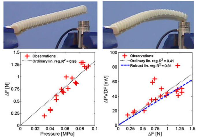
Fig. 11. Force-sensing calibration. Top left—initial free configuration. Top right—upon actuation the bi bellows presses against the force sensor. Bottom left—contact-force norm,  $\Delta F$ , as a function of the actuation pressure. Bottom right—PVDF response,  $\Delta PVDF$ , as a function of  $\Delta F$ , the contact-force norm. Ordinary and robust linear-regression trend-lines are used.
