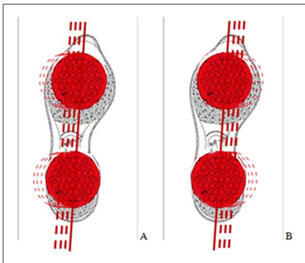
**Figure 2.** Different configurations of the biomechanical shoe device: Six medial (M 0.4, M 0.8, M 1.2) and lateral (L 0.4, L 0.8, L 1.2) axes were defined as 0.4, 0.8, and 1.2 cm medial (dashed lines in B) and lateral (dashed lines in A) deviation of the biomechanical elements from the neutral (N 0.0) sagittal axis (solid line), respectively.
