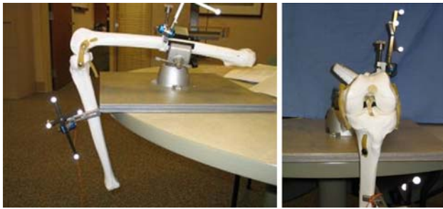
Fig. 5 Experimental setup with optical trackers attached (Sawbones)
