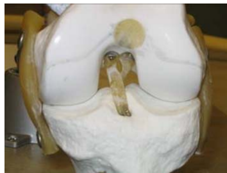
Fig. 4 Knee model with Sawbones and artificial ligaments
