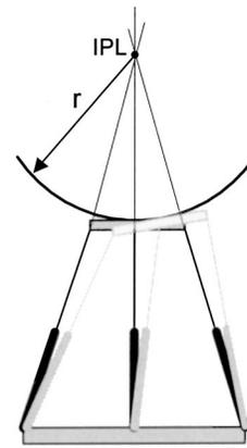
Fig. 11 The path of the moving platform on a sphere centered at IPL
