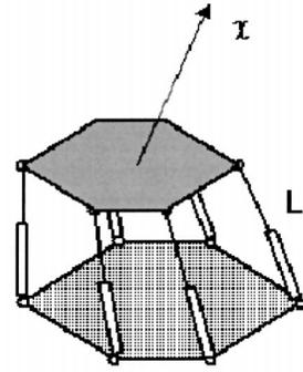
Fig. 1 Gough-Stewart platform, the lines  $L_i$  and the resulting twists
