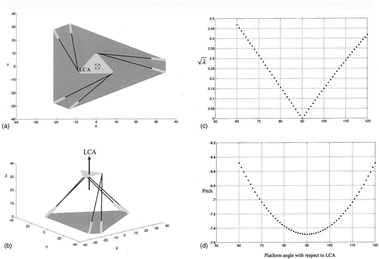
Fig. 3 (a) Fichter's singularity—90 deg rotation of the moving platform about the Z axis, top views; (b) Fichter's singularity—90 deg rotation of the moving platform, from home position, about the Z axis: isometric views; (c)  $\sqrt{\lambda}$  as a function of the moving platform rotation angle about the Z axis. (d) Values of the closest linear complex's pitch as a function of the moving platform rotation angle about the Z axis.
