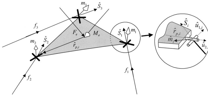
Fig. 9 Force and moment transmitted to the moving platform
