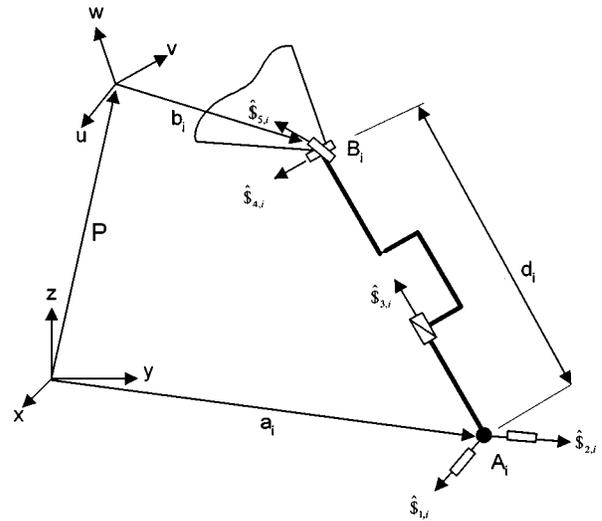
Fig. 8 Equivalent kinematic structure of the UPU robot's limb
