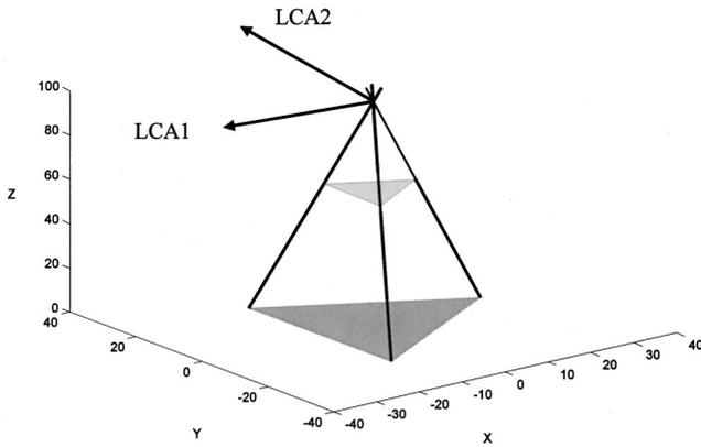
Fig. 10 3-UPU with two zero-pitch linear complexes
