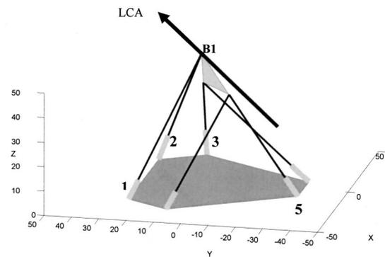
Fig. 5 Type 3c singularity with four line-1,2,3,5-intersect at vertex B1
