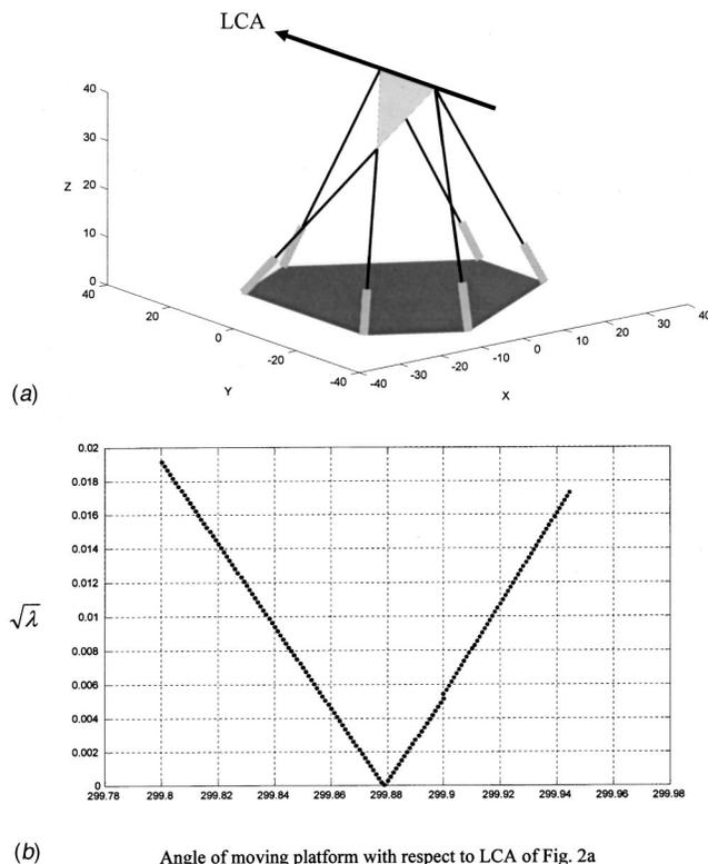
**Fig. 2 (a)** Hunt's singularity—two limbs and the moving platform are coplanar; **(b)**  $\sqrt{\lambda}$  as function of the moving platform rotation angle,  $\alpha$ , about the LCA axis of Fig. 2(a)
