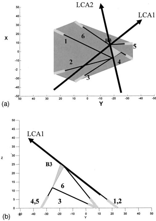
Fig. 6 (a) Type 4d singularity where lines LCA1 and LCA2 cross the plane spanned by L1 and L2, vertex B3 joining L5 and L6 and intersect a line along limb 4: top view; (b) Type 4d singularity (LCA2 not shown for clarity): side view.
